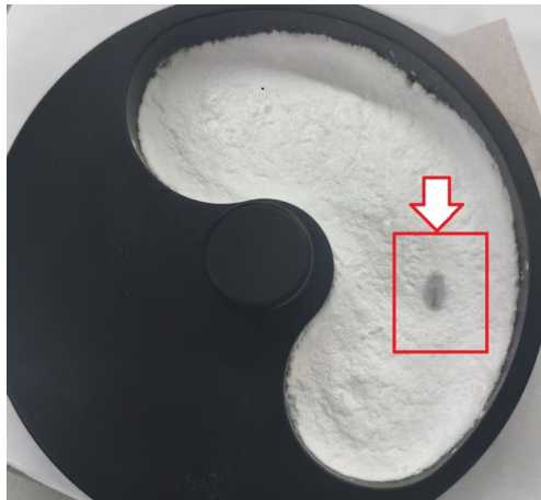
图7 硬脂酸在设备I样品盘中出现熔化现象 Fig. 7 Melting phenomenon of stearic acid observed in sample cell of Instrument I
